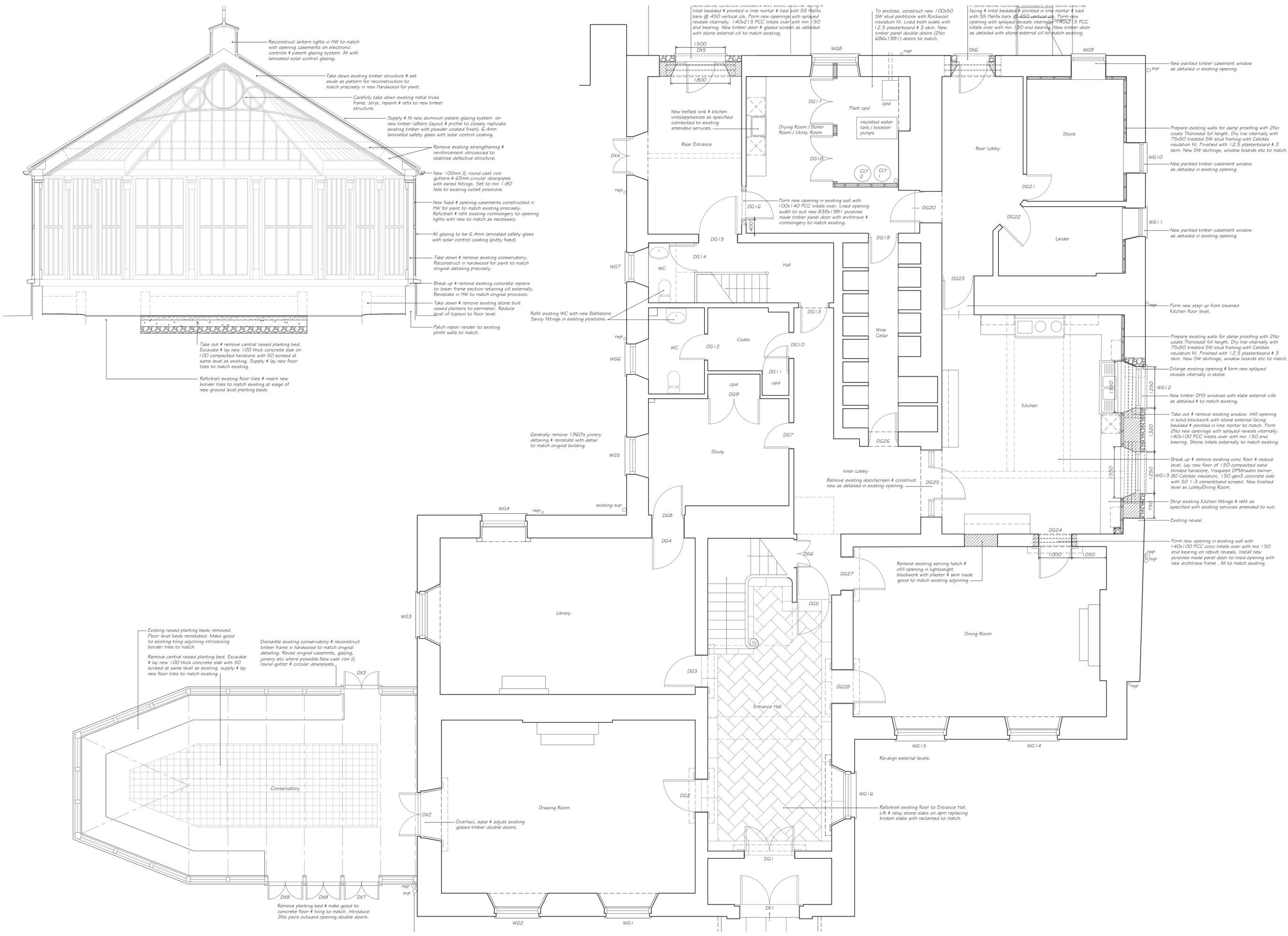
Reconstruct lantern lights in HW to match with opening casements on electronic controls & patent glazing system. All with laminated solar control glazing.
